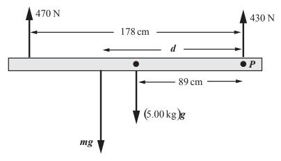
The forces responsible for a counterclockwise torque about an axis through your feet (point P) and perpendicular to the page are your weight and the weight of the board. The only force causing a clockwise torque about this axis is the 470 N force exerted by the scale under your head. Apply  $\sum \vec{\tau} = 0$  about an axis through your feet and perpendicular to the page:
