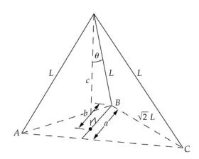
Letting  $F_{\rm C}$  represent the compressional force in a leg of the tripod, apply  $\sum \vec{F} = 0$  to the apex of the tripod:
