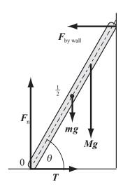
(a) Apply  $\sum \vec{\tau} = 0$  about an axis through the bottom of the ladder:
