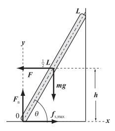
To find the force required to pull the ladder away from the wall, apply  $\sum \vec{\tau} = 0$  about an axis through the bottom of the ladder:
