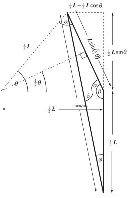
Apply  $\sum \vec{\tau} = 0$  to the beam about an axis through the bearing point to obtain:
