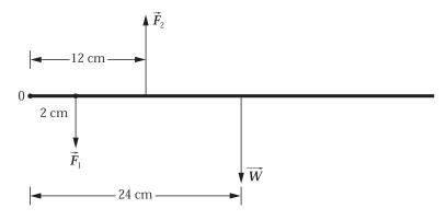
(a) Letting the upward force exerted by the fencer's hand be F, apply  $\sum_{v} F_{v} = 0$  to the epee to obtain:
