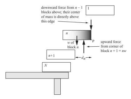
(a) and (b) Noting that the line of action of the downward forces exerted by the blocks above the *n*th block passes through the point P, resulting in a lever arm of zero, apply  $\sum \tau_P = 0$  to the *n*th brick to obtain:
