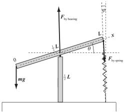
The pictorial representation directly above shows the forces acting on the beam when it is in static equilibrium. The pictorial representation to the right is an enlarged view of the right end of the beam. We'll use this diagram to determine the length of the stretched spring.
