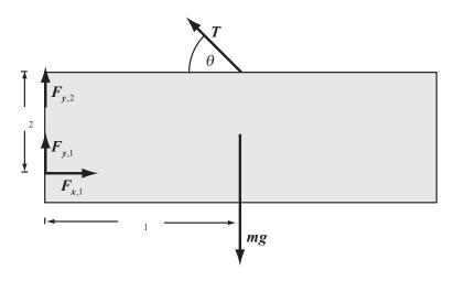
(a) Apply  $\sum \vec{\tau} = 0$  about an axis through the lower hinge and perpendicular to the plane of the page:
