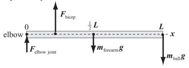
Apply  $\sum \vec{\tau} = 0$  about an axis through  $\ell F_{\text{bicep}} - \frac{1}{2} L m_{\text{forearm}} g - L m_{\text{ball}} g = 0$ the elbow and perpendicular to the plane of the diagram:
