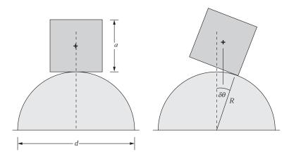
If the displacement of the cube's center of mass is less than that of the point of contact, the torque about the point of contact is a restoring torque, and the cube will return to its equilibrium position. If, on the other hand,  $(a/2) \delta\theta > (d/2) \delta\theta$ , then the torque about the point of contact due to mg is in the direction of  $\delta\theta$ , and will cause the displacement from equilibrium to increase. We see that the minimum value of d/a for stable equilibrium is
