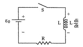
In this circuit,  $\epsilon_0 = 12$  V, R = 6.0  $\Omega$ , and L = 0.48 H. The switch is closed at time t = 0. At time t = 0.25 s, the rate of Joule heating is approximately
