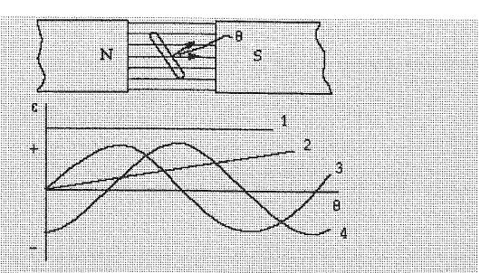
A simple generator consists of a single rectangular loop of wire rotating between two magnetic pole faces as shown. Which curve in the graph correctly represents the emit cas a function of the angle between the normal to the plane of the coil and the direction of the magnetic field?
