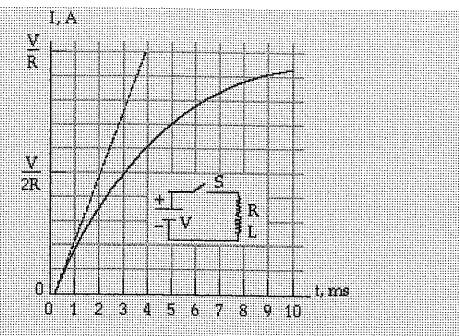
The growth of current in the inductive circuit in the inset diagram is represented by the curve in the graph. The broken line is tangent to the curve at the origin. The time constant of the circuit is approximately
