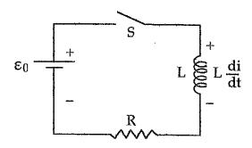
In this circuit,  $\epsilon_0$  = 12 V, R = 6.0  $\Omega$ , and L = 0.48 H. The switch is closed at time t = 0. At time t = 0.25 s, the rate at which the battery is supplying power is approximately
