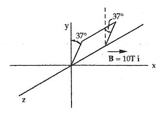
A rectangular surface of area 1.0 m<sup>2</sup> is hinged along the z axis and makes an angle of 37° with the yz plane. If the local magnetic field is 10 Ti, the magnetic flux through this surface is
