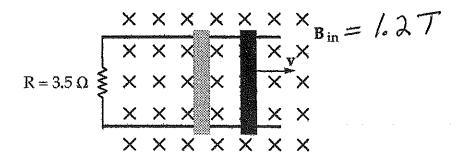
A wire rod rolls with a speed of 8.0 m/s on two metallic rails, 30 cm apart, that form a closed loop. The magnitude and direction of the current induced in the resistor R are
