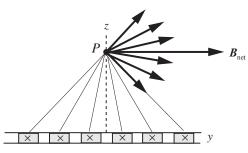
(c) The magnetic field is in the +y direction. This result follows from the same arguments that were used in (a) and (b).
