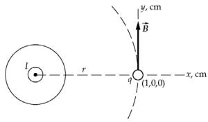
Express the magnetic force acting on  $\vec{F} = q\vec{v} \times \vec{B}$  the electron:
