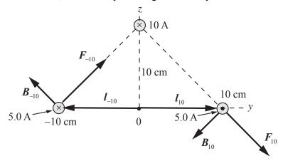
(a) The net torque about the x axis is the sum of the torques due to the forces  $\vec{F}_{10}$  and  $\vec{F}_{-10}$ :
