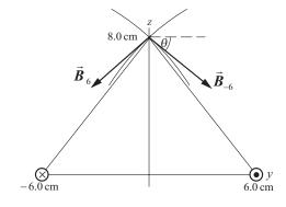
Noting that the y components add to zero, express the resultant magnetic field at z = +8.0 cm:
