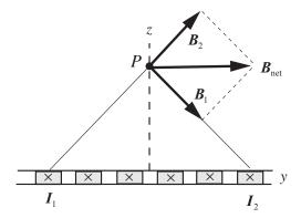
(b) The vertical components of the field cancel in pairs. The magnetic field is in the +y direction.
