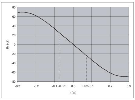
Inspection of the table reveals that the slope of the graph of  $B_z$ , evaluated at z = 0, is -337 G. 1% of this value corresponds approximately to -0.075 m < z < 0.075 m -0.25R < z < 0.25R .
