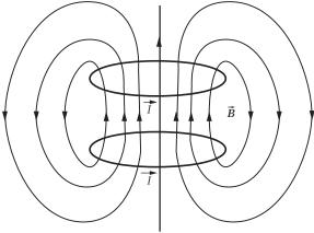
(b) The field-line sketch is shown below. An assumed direction for the current in the coils is shown in the diagram. Note that the field lines never begin or end and that they do not touch or cross each other. Because there are an uncountable infinity of lines, only a representative few have been shown.
