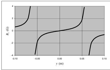
27 •• The current in the wire at y = -6.0 cm is in the -x direction and the current in the wire at y = +6.0 cm is in the +x direction. Find the magnetic field at the following points on the y axis: (a) y = -3.0 cm, (b) y = 0, (c) y = +3.0 cm, and (d) y = +9.0 cm.
