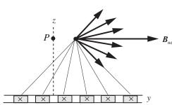
(d) Below the sheet the magnetic field points to the left; i.e., in the -y direction. The vertical components cancel in pairs.
