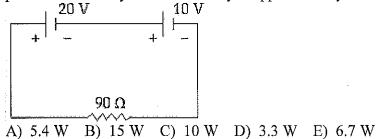
2. The current through the battery in the figure is approximately
