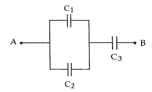
You connect three capacitors as shown in the diagram. The effective capacitance of this combination when C  $_1$  = 5.0  $\mu$ F, C $_2$  = 4.0  $\mu$ F, and C $_3$ = 3.0  $\mu$ F is approximately
