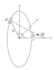
(a) Express the differential gravitational field at a distance x from the center of the ring in terms of the mass of an elemental segment of length dL:
