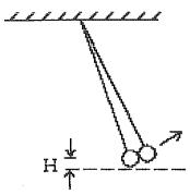
Two identical masses are hung on strings of the same length. One mass is released from a height h above its free-hanging position and strikes the second mass; the two stick together and move off. They rise to a height Higiven by
