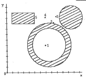
The mass of the rectangle in the figure is M, the mass of the ring is M, and the mass of the circle is 3M. The center of mass of the system with respect to the origin O is located at point
