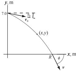
(a) Use a constant-acceleration equation to relate the y coordinate of the ball to its time-in-flight:
