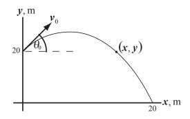
(a) Using constant-acceleration equations, express the x and ycoordinates of the rock as functions of the time into its flight:
