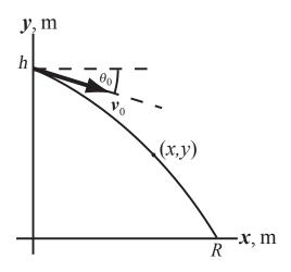
(a) Using a constant-acceleration equation, express the x coordinate of the hammer as a function of time:
