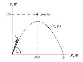
(a) Use a constant-acceleration equation to express the x coordinate of the ball as a function of time:
