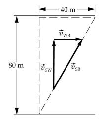
$$\frac{v_{\text{WB}}}{v_{\text{SW}}} = \frac{40 \,\text{m}}{80 \,\text{m}}$$
