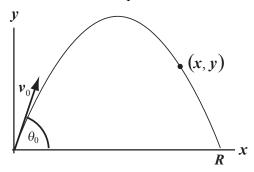
(a) Using a constant-acceleration equation, express the x coordinate of a bullet in flight on the moon:
