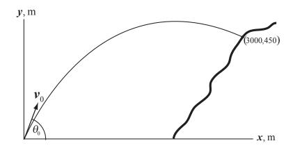
(a) Using a constant-acceleration equation, express the vertical displacement of the projectile as a function of its time of flight:
