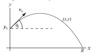
Use constant-acceleration equations to express the x and y components of a molecule of water in the stream:
