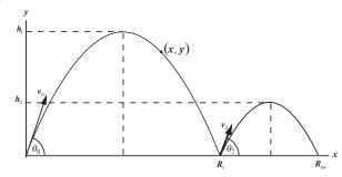
(a) Use constant-acceleration equations to express the x and y coordinates of the tennis ball along its first parabolic trajectory as functions of time:
