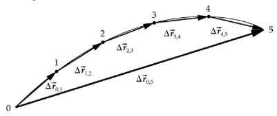
Suppose we take a trip along some path and consider the trip as a sequence of many very small displacements. The net displacement is the vector sum of the very small displacements, and the total distance traveled is the sum of the magnitudes of the very small displacements. That is,
