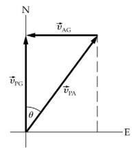
(a) Referring to the diagram, relate the heading you must take to the wind speed and the speed of your plane relative to the air:
