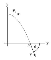
Express the direction of the velocity vector when the projectile strikes the ground:
